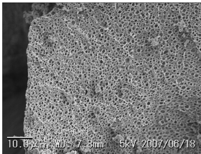
Figure 2. SEM image of the tannin gel particle surface.
